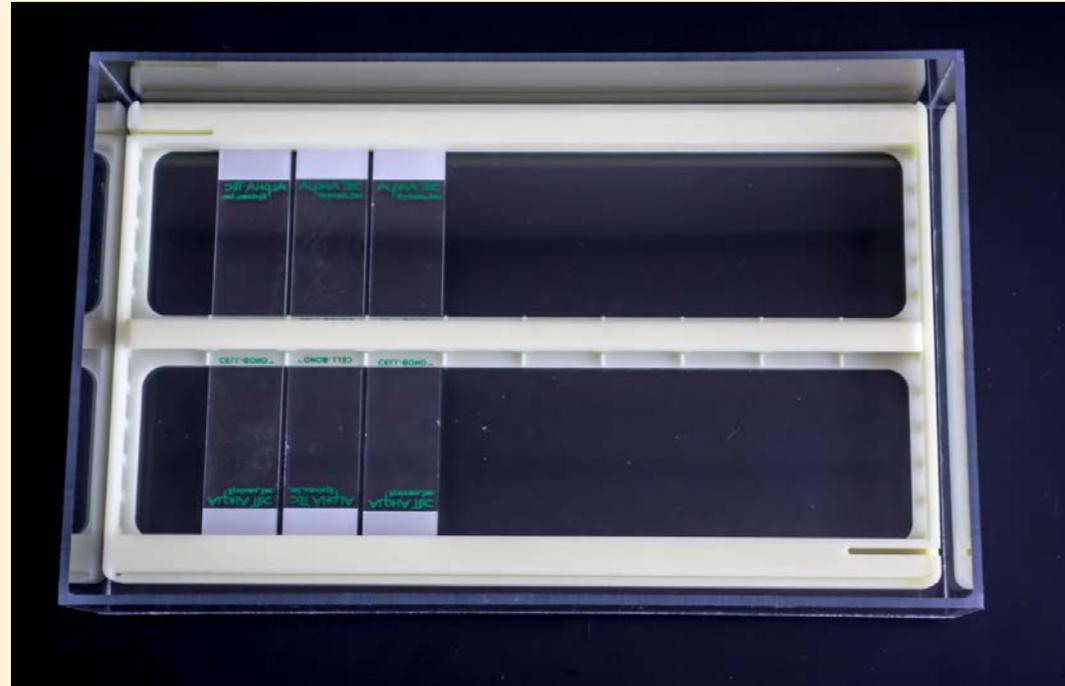
**TIP : ACD EZ Batch slide processing tray is easy and convenient for loading multiple slides for washing steps.**
