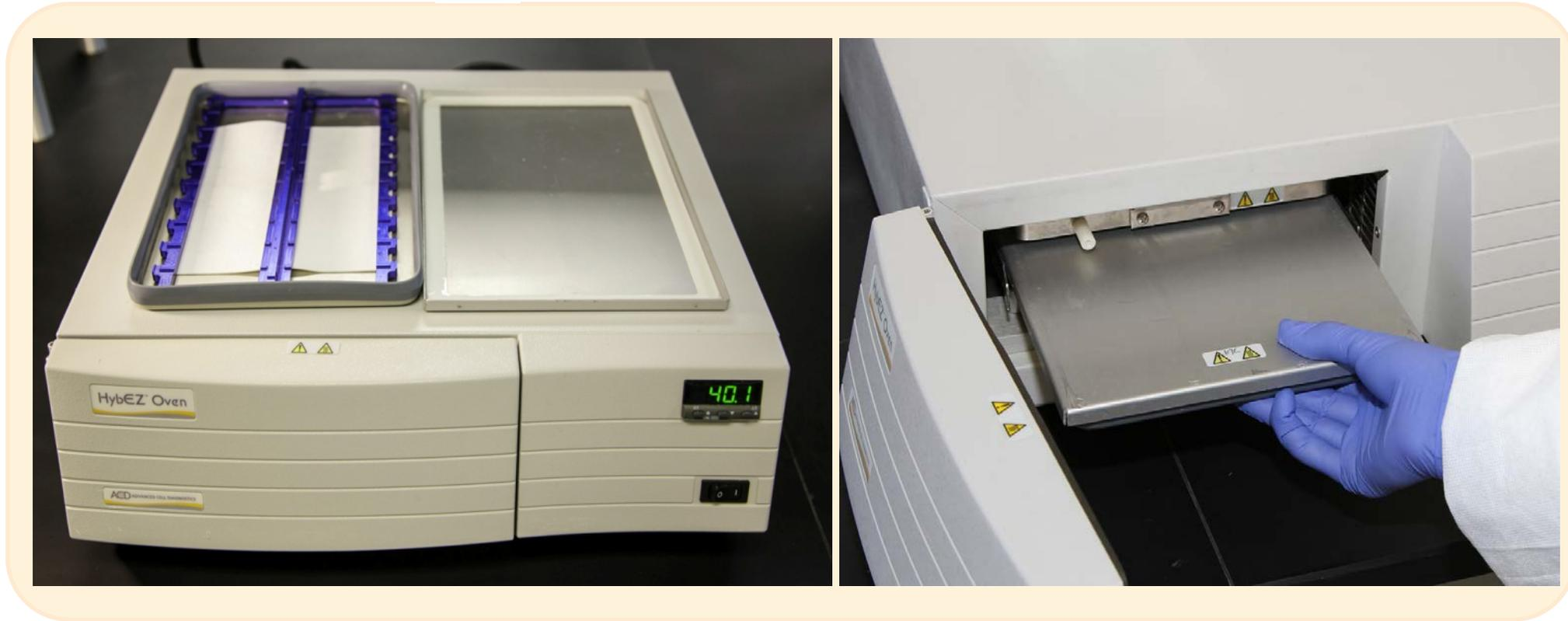
***TIP: HybEZ oven is required as it provides both temperature and humidity control, necessary to obtain optimal RNAscope results***
