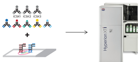
Figure 1. Graphical schematic of the 3-step procedure to acquire RNA and protein co-detection data with IMC
